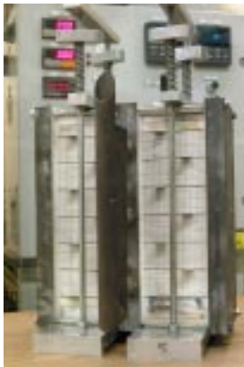
SOFCo and Cummins have teamed up to develop a 4-kW fuel cell for the SECA program. This photo shows SOFC's 60-cell solid oxide fuel cell unit.
