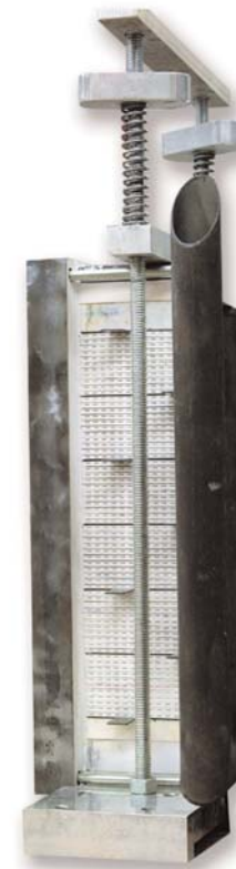
Solid oxide fuel cells (SOFC) use hard ceramic electrolytes instead of a liquid and operate at high temperatures. Pictured is a 60-cell SOFC stack developed by SOFCo.
