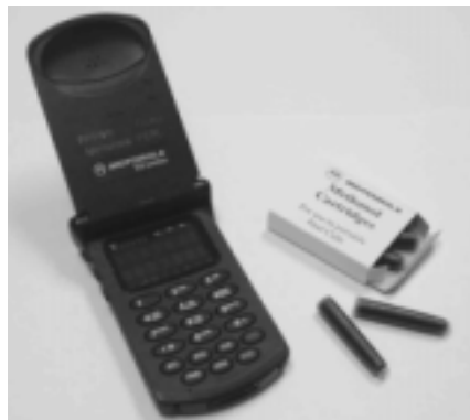
Motorola is developing fuel cell-powered cell phones that refuel quickly with cartridges of methanol.
